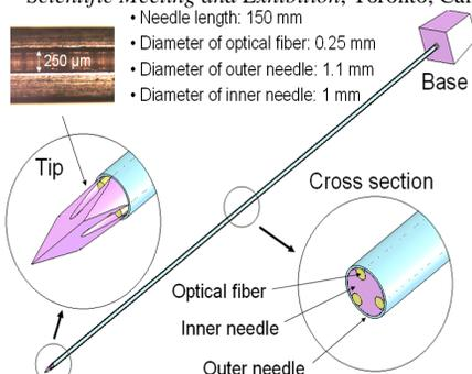
Figure 1. CAD Model of fabricated 18-ga needle, and magnification of one of the needle grooves, 250- $\mu\text{m}$  deep and wide, machined using EDM.
