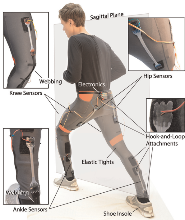
Fig. 1. Soft strain sensors were placed at each lower limb joint to capture motion in the sagittal plane. In the case of the knee and ankle sensors (insets on left) webbing directed motion over the joint.
