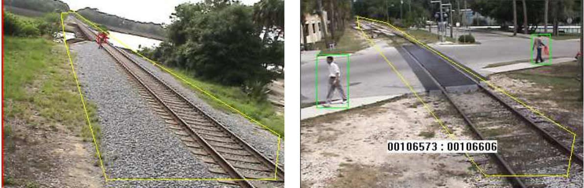
Figure 2. Detecting entry into the danger zone. A danger zone is defined through a GUI and objects are warned as they enter the danger zone. The bounding box of individuals turn red as they enter the polygon defining the danger zone.
