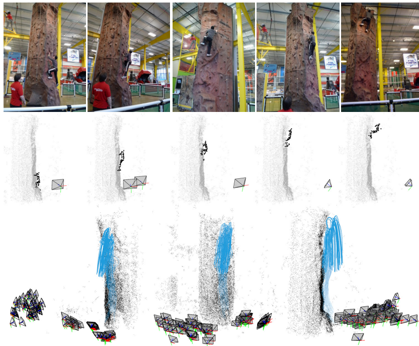
Fig. 4. Results of the rock climbing scene. Top row: sampled image input, second row: five snapshots of 3D reconstruction in different views, and bottom row: reconstructed trajectories (blue line) in different views.
