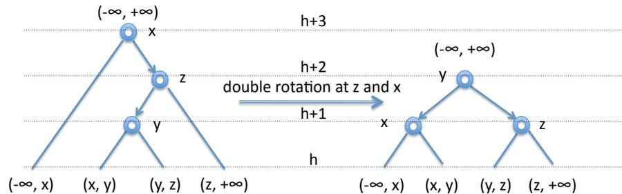
In that case, a left rotation alone will not restore the invariant (see Exercise 1). Instead, we apply a so-called *double rotation*: first a *right rotation* at  $z$ , then a *left rotation* at the root. When we do this we obtain the picture on the right, restoring the height invariant.
