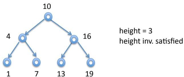
If we insert a new element with a key of 14, the insertion algorithm for binary search trees without rebalancing will put it to the right of 13.
