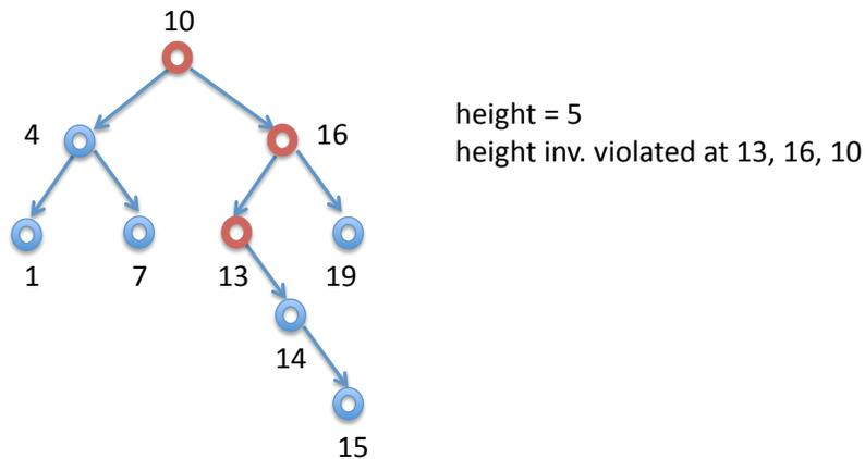
All is well at the node labeled 14: the left subtree has height 0 while the right subtree has height 1. However, at the node labeled 13, the left subtree has height 0, while the right subtree has height 2, violating our invariant. Moreover, at the node with key 16, the left subtree has height 3 while the right subtree has height 1, also a difference of 2 and therefore an invariant violation.
