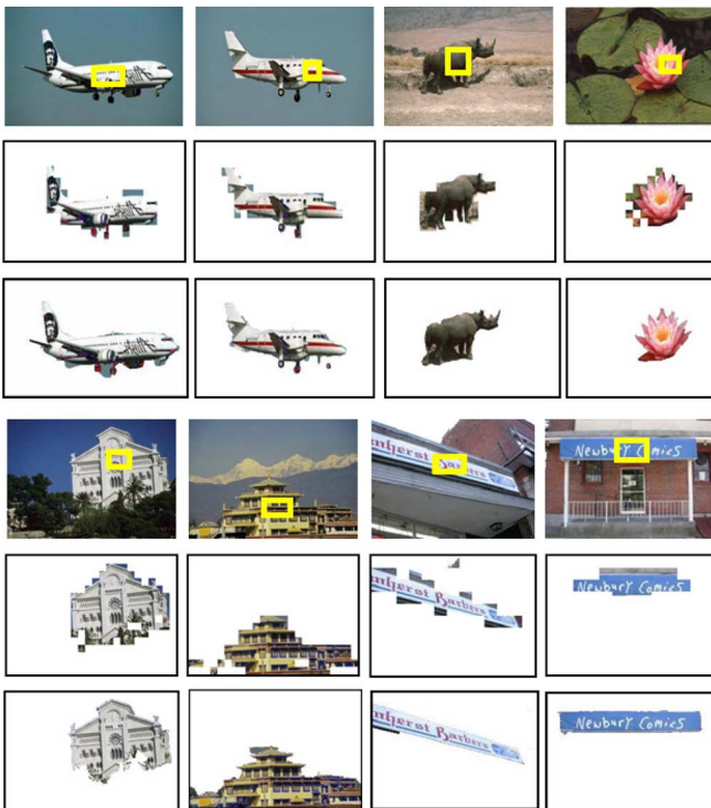
Fig. 8. Comparison between SmartLabel [13] and SmartLabel-2. In two groups of three rows. The first row shows input images with ROIs. The second row shows results by SmartLabel. The third row shows results by SmartLabel-2. Two merits of SmartLabel-2 compared to SmartLabel: 1) smooth object boundaries instead of zigzag lines and 2) less misclassified patches.
