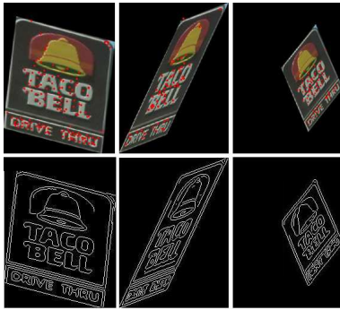
Figure 3: Synthesized views of the Taco Bell sign and extracted keypoints and edges for these views.
