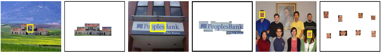
Figure 2: Examples of SmartLabel. The user loosely drags a rectangle inside an object. The object and others at different locations if any are then extracted automatically. Left is the input image with user specified ROI and right is extracted object region(s) using SmartLabel.
