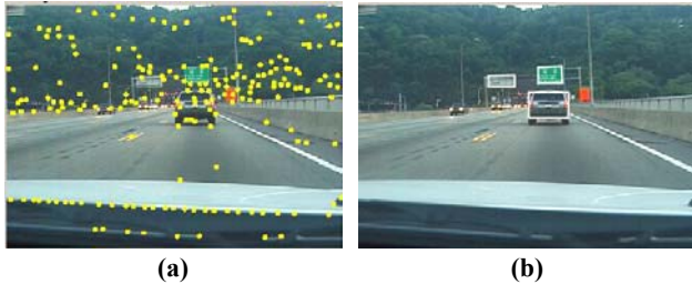
Figure 9. False positive examples of road sign localization.
