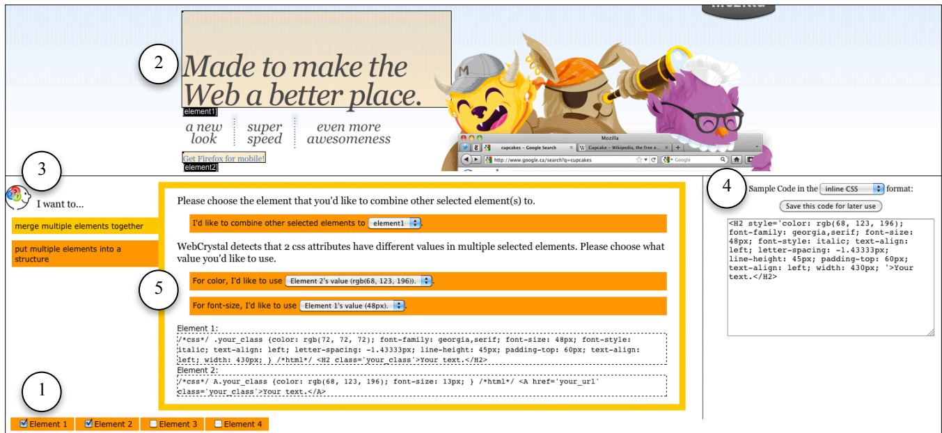
Figure 6: The interface for combining multiple elements. (1) the elements stored to be combined. (2) elements selected in (1) being highlighted in the web page in brown boxes. (3) the two commands of how to combine the elements. (4) the generated code for all selected elements merged together. (5) when an attribute is in multiple elements with conflicting values, the user can select which one to use.
