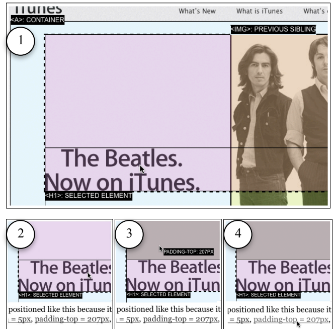
Figure 3: When answering position questions, WebCrystal (1) highlights the container and the siblings of a selected element, and (3) allows user to inspect blank areas around the element on the web page or (4) inside the textual explanation using the mouse.
