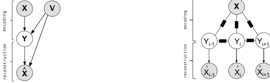
Figure 2: Graphical model representations of CRF autoencoders. Left: A general CRF autoencoder model. In the encoding part of the model, the observed variables \mathbf{X} , \mathbf{V} generate \mathbf{Y} . In reconstruction, \mathbf{Y} , \mathbf{V} generate \hat{\mathbf{X}} . The internal structure of \mathbf{X} , \mathbf{Y} , \hat{\mathbf{X}} is not shown. Right: An instantiation of the CRF autoencoder model for POS tagging, represented as a hybrid graphical model showing the first-order Markov dependencies among elements of the hidden structure \mathbf{Y} , the factor cliques used in the CRF encoder, and the independent generation of the atomic parts of \hat{\mathbf{X}} .
