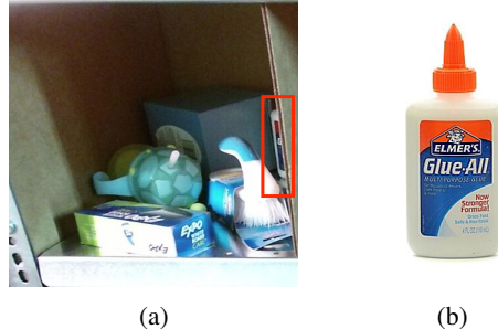
Fig. 1: A typical scene from a warehouse picking task. Here, we have access to the list of objects in the bin, their 3D models and that of the shelf as well. (a) An image of the shelf-bin from which we are required to identify and localize the Elmer’s glue bottle, marked by a red bounding box. (b) An image of the Elmer’s glue bottle that needs to be localized.
