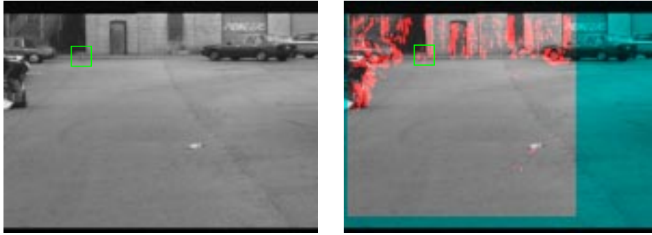
Figure 6: An image of a parking lot, and the obstacle image. Obstacles identified are marked in red. The blue-ish region was not processed.
