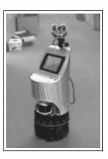
**Figure 1**: *Florence Nightingale*, the prototype nursing home robot used in these experiments.
