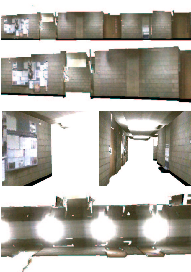
Figure 3: Views of a compact 3D texture map built in real time with an autonomously exploring robot.
