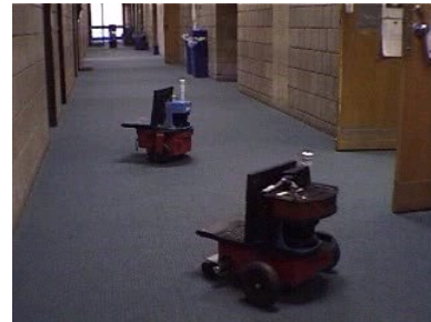
Figure 1: The laser tag robots are equipped with light-emitting devices and receivers.
