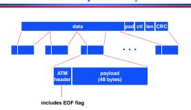
Pertinent part: Packets are spread across multiple ATM cells. Each packet is delimited by EOF flag in cell.
