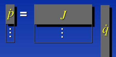
Underdetermined linear system Can solve for  $\dot{q}$
