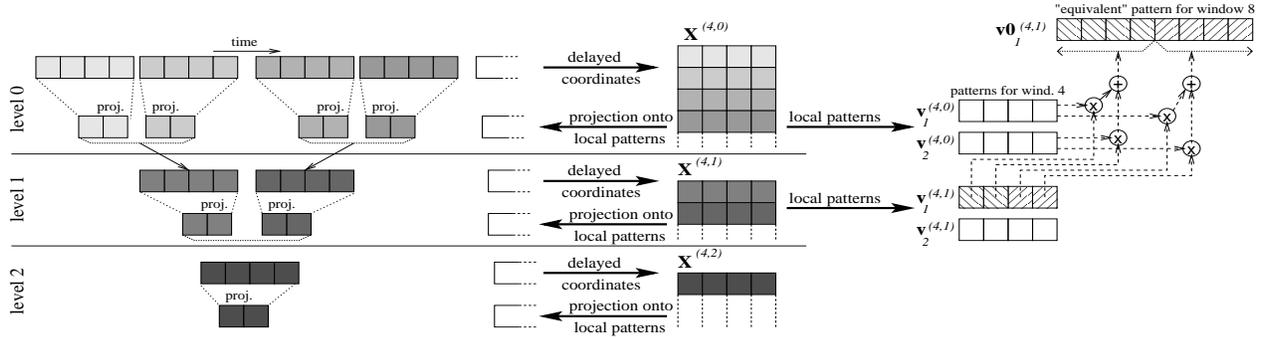
Figure 6: Multi-scale pattern discovery (hierarchical,  $w_0 = 4$ ,  $W = 2$ ,  $k = 2$ ).
