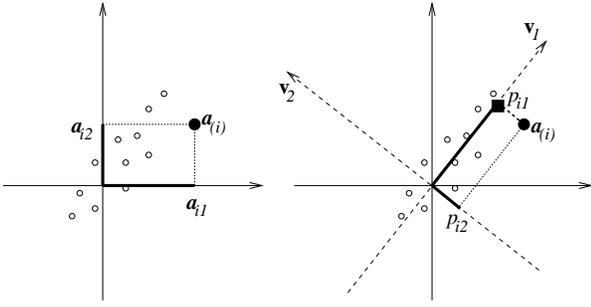
**Figure 3: Illustration of SVD (for dimension  $n = 2$ ), with respect to row space. Each point corresponds to a row of the matrix  $\mathbf{A}$  and  $\mathbf{v}_j$ ,  $j = 1, 2$  are the left singular vectors of  $\mathbf{A}$ . The square is the one-dimensional approximation of  $\mathbf{a}_{(i)}$  by projecting it onto the first singular vector.**
