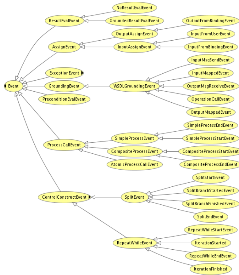
Fig. 1. Event types taxonomy. Only selected classes are displayed, particularly, specific ExceptionEvent types are not shown (see Section 4) and only some ControlConstructEvent types are shown.
