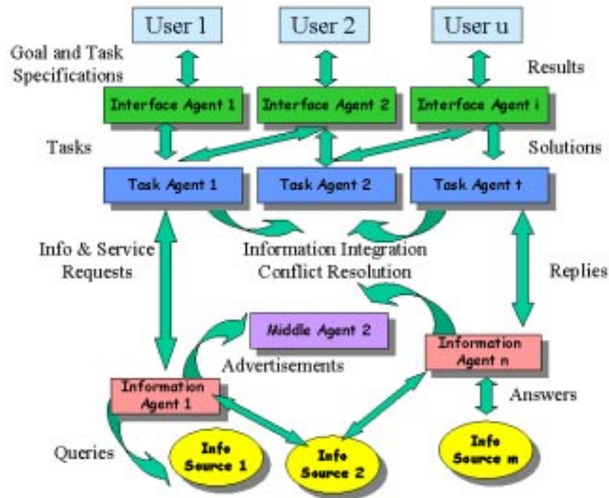
Fig. 2. The RETSINA Functional Architecture
