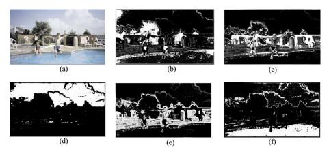
Fig. 4. Cluster Probability Maps corresponding to different clusters (j) obtained from the soft clustering of the input image. (a) Input color image. (b) j = 1. (c) j = 2. (d) j = 3. (e) j = 4. (f) j = 5.
