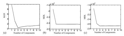
Fig. 3. Model selection results on the synthetic data. (a) KLD-based model selection on the synthetic data. KLD correctly favors three components. (b) A typical run of MDL incorrectly favors two components. (c) Another typical run of MDL correctly favors three components.
