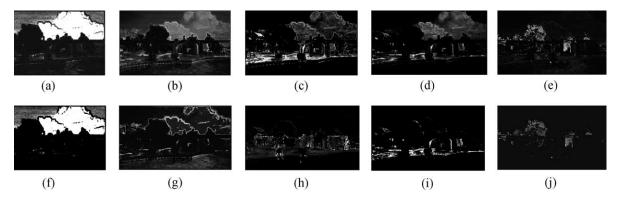
Fig. 6. For the input image shown in Fig. 4(a), (a)–(e) Original Class Density Maps corresponding to the class sky, water, skin, sand/soil, and tree/grass. (f)–(j) Corresponding Constrained Class Density Maps.
