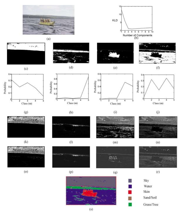
Fig. 9. (a) Input color image. (b) KLD-based model selection favors four components. (c)-(f) Cluster Probability Maps for each of the four clusters. (g)-(j) Corresponding Class posterior distributions. (k)-(n) Class Density Maps for sky, grass/tree, skin, and water, respectively. (o)-(r) Corresponding Constrained Density Maps. (s) MAP Discriminative result showing the semantic classification of various image regions.
