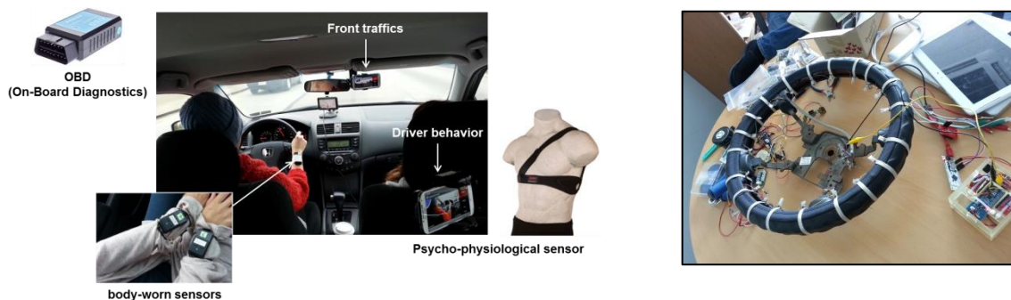
Figure 15. Sensors in a field study (left) and a prototype sensing steering wheel (right, via collaboration with UNIST).
