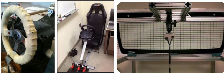
Figure 16. Prototypes of in-car feedback systems: haptic steering wheel (left, with KAIST), haptic driver seat (center, with AT&T), and laser projective display for car windshield (right, with GM).
