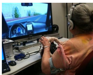
Figure 9. Simulated driving test-bed with multisensory cues and wearable sensors.
