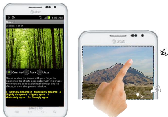
Figure 8. In the main study, an Android Application provides combinational effects of visual, auditory, and haptic cues which vary according to textures on the images where the user's finger is touching and hovering.
