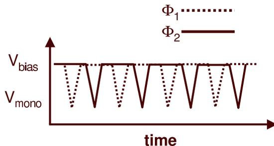
Figure 7: Two-phase clocking scheme used for series latches.
