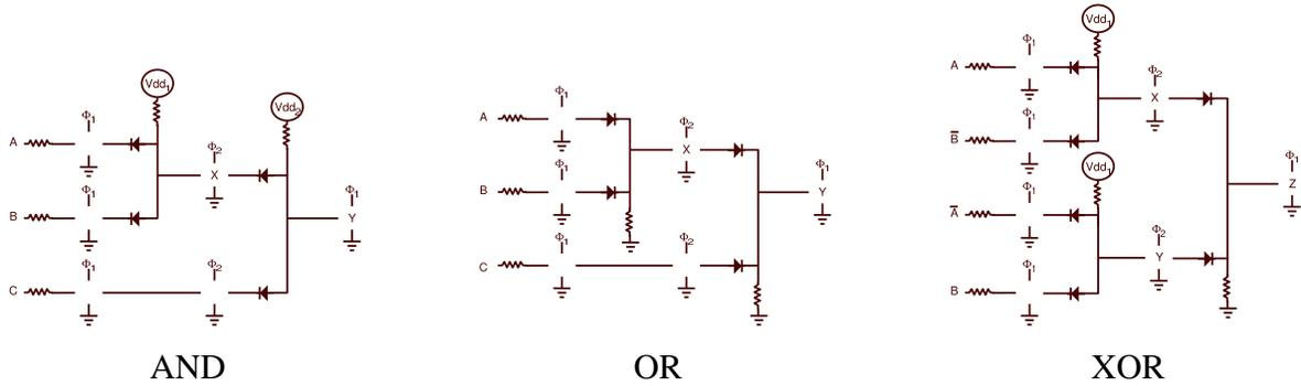
Figure 9: *AND, OR, XOR circuits using diode-resistor logic and intermediate molecular latches.*
