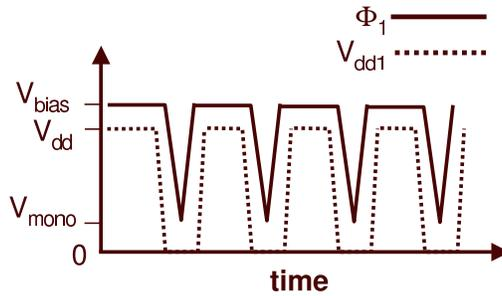
Figure 11: Clocking scheme used for  $V_{dd}$ .
