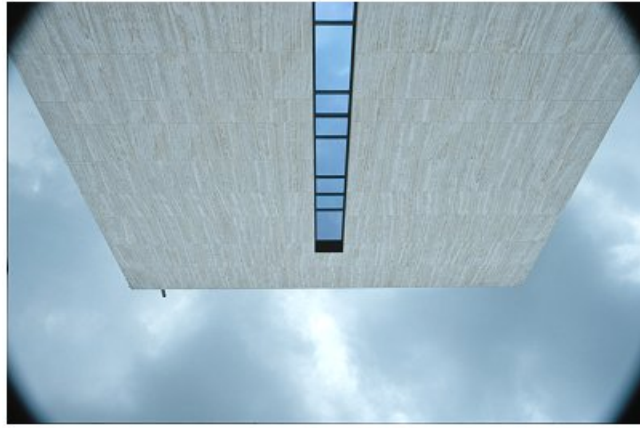
Figure 7. A typical case of mechanical vignetting. (Distagon 28/2 @ f/11 + Contax metal hood #3)
