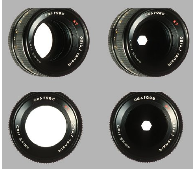
Figure 2. The Planar 50/1.4 at f/1.4 (left) and f/5.6 (right) seen from the optical axis (top) and from the semifield angle (bottom).
