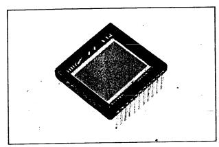
CCD222 488X380 Element Area Image Sensors are also included in Fairchild Weston's series of solid-state television camera systems.
