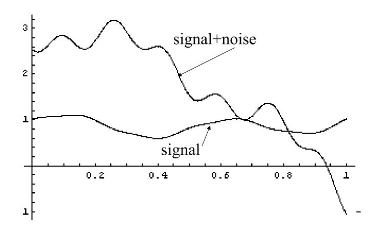
(3) when the signal (but not the noise) is modulated this is how the synchronous rectifier output looks:
