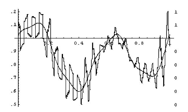
heavier filtering would faithfully restore the original signal, distorted (under favorable conditions only slightly) by the noise that happens to be in the frequency and phase band accepted by the process
