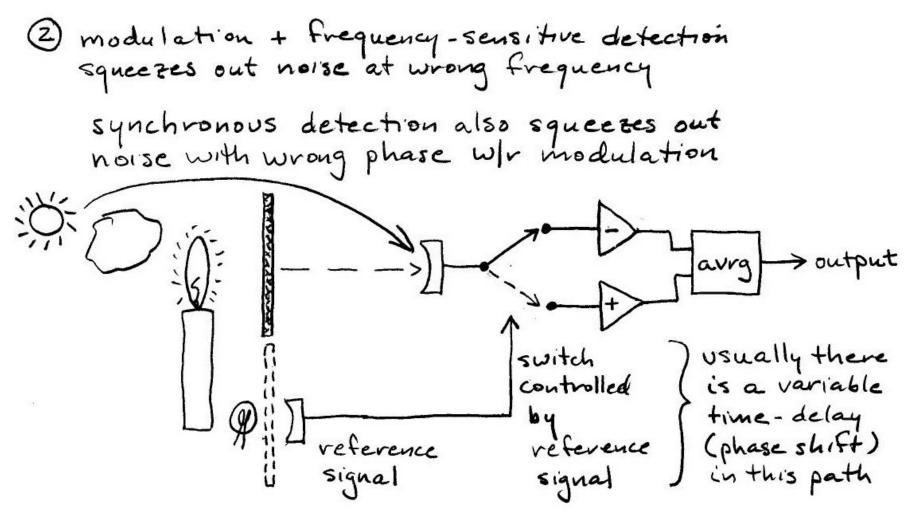
the reference signal may drive the modulator, or the modulator may be "free running" and the reference signal obtained by monitoring it (as shown here), or it can (with difficulty) be extracted from the signal itself
