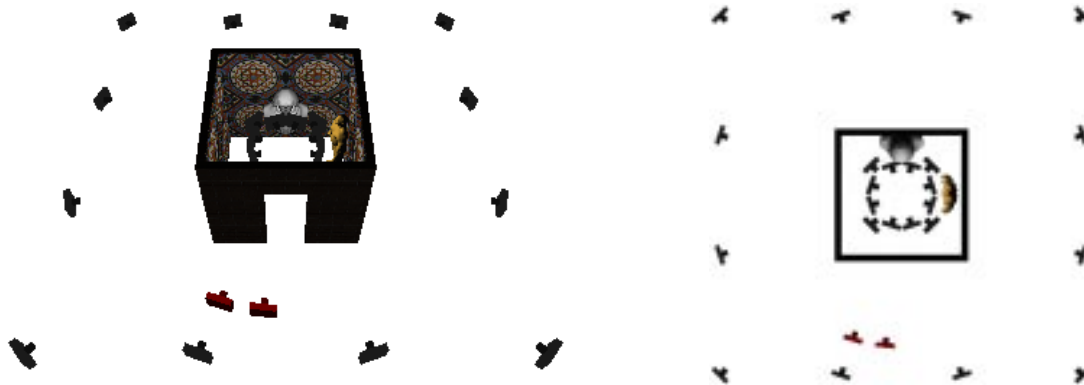
Fig. 10: Cameras for the building scene. Cameras were placed in both the interior and exterior of a building to enable simultaneous, complete reconstruction of its exterior and interior surfaces. The viewpoints used by the carving algorithm are shown in gray; the two red cameras correspond to the building’s views in Figs. 12(a)-(d).
