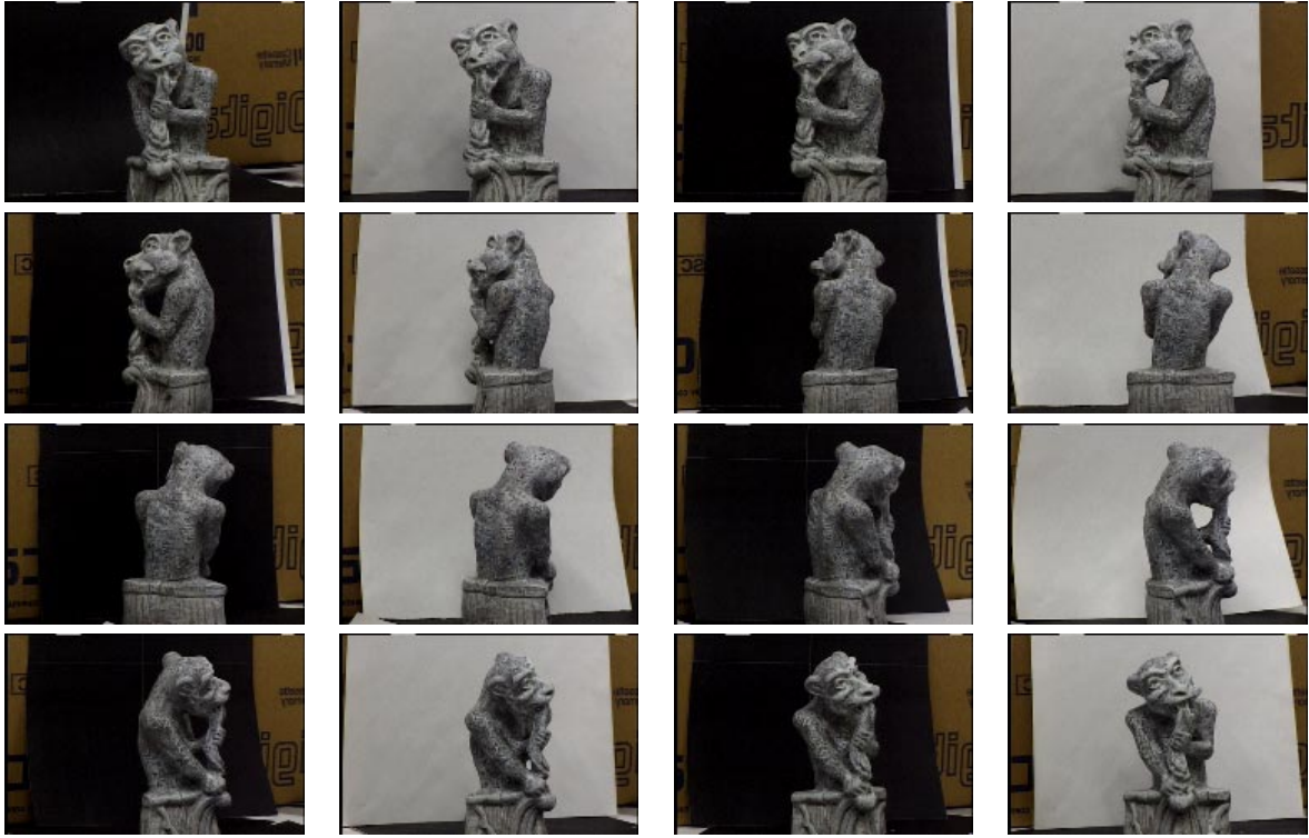
Fig. 8: A sequence of sixteen 486x720 RGB images of a gargoyle stone sculpture. The sequence corresponds to a complete rotation of the object in front of a stationary camera, performed in 22.5 degree increments.
