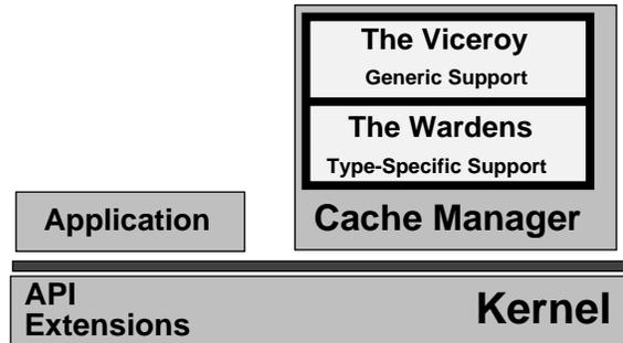
This figure illustrates the architecture of an Odyssey client. Odyssey applications make use of the Odyssey API extensions along with the operating system's API. Operations on Odyssey objects are redirected by the kernel to the cache manager, which is at user level for ease of implementation. The cache manager is split into two logical pieces: the viceroy, providing generic support, and a set of wardens, each supporting a single type.
