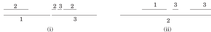
Fig. 3. An example of compression in one dimension. (i) An input with six prefix ranges, and (ii) an optimal solution using four prefix ranges.
