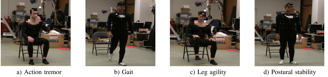
Fig. 1. In this figure, four frames of the motion capture session are shown. The subjects went through various motor tests: a) action tremor, b) gait, c) leg agility and d) postural stability. All the patients wore a body leotard with 60 reflective markers attached to it and performed various motor tasks. A trained clinician was monitoring them and assigning the scores for various motor components.
