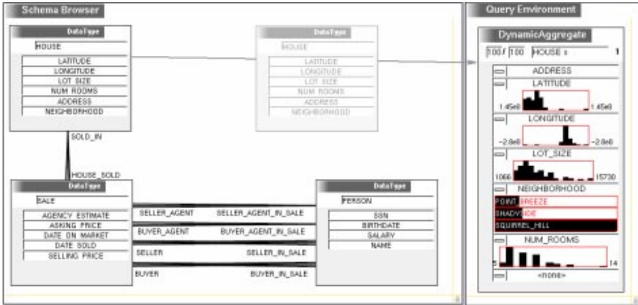
Figure 1: Left: Entity-Relationship diagram for the Real Estate domain. Right: The House data type has been dragged to QueryEnvironment (VQE), which creates a dynamic aggregate containing all (100) houses in the dataset being explored. Histogram sliders have also been dropped on most attributes, but no filtering has been done, so all 100/100 houses are selected.
