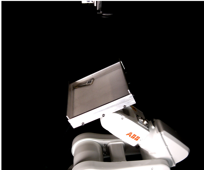
Figure 3.6: Tray tilting experimental setup. The robot tilts the aluminum tray in various directions, and the camera records the resulting pose of the object inside.
