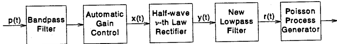
Figure 3-3: Block diagrams of (a) the original auditory-nerve model as specified by Colburn (1973) and (b) the new version of the auditory-nerve model used for this work.
