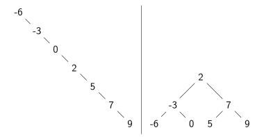
The height of the left tree is 7, while the height of the right tree is only 3. Say we want to access the element 9. In the left tree, we need to travel down 7 levels, while on the right we only need to go down 3. Remember that we have to do a comparison at each level, so we'd like our trees to be as short as possible.
