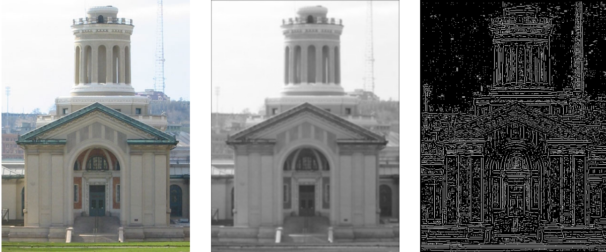
Figure 5: Hammerschlag Hall: original image (left), blurred with the mask (middle), and after running edge detection (right). See text for mask values.
