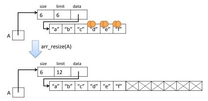
After the resize, exactly half the array is full, so our data structure invariant for tokens doesn't require us to have any tokens in reserve. This means that the data structure invariant is preserved in this case as well.
