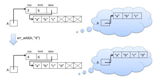
The images to the left above represent how the data structure is actually stored in memory, and the images in the thought bubbles to the right represent how the client of our array library can think about the data structure and after a arr\_add operation.
