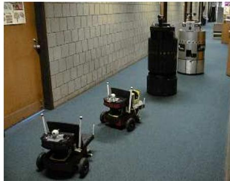
Figure 4: Coordinated deployment of heterogeneous robots
