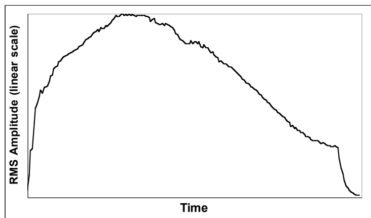
Figure 7. A typical trumpet amplitude envelope (an Ab 4 , mezzo forte , from an ascending scale of tongued quarter notes). Note the rapid decay at the end.
