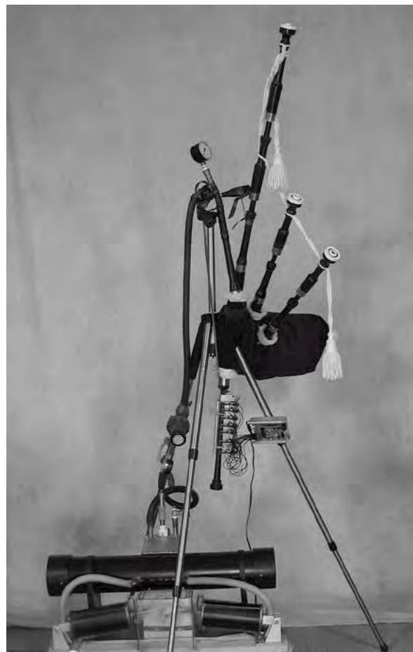
Figure 3. McBlare, Carnegie Mellon's robotic bagpipe player.
