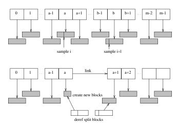
Figure 2. Deleting samples from a Sequence.
