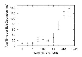
Figure 3. These performance measurements show that the time to perform one editing operation, while small, is affected by the total size of the file, probably due to less disk caching.
