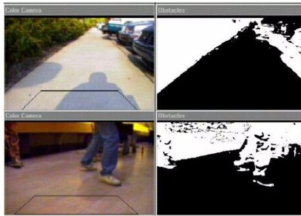
Fig 4.48 Examples of adaptive floor plane extraction. The trapezoidal polygon identifies the floor sampling region.
