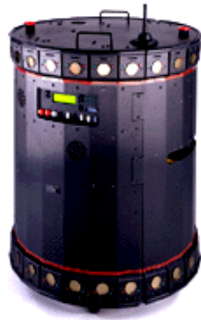
Fig 2.25 The Nomad XR4000 from Nomadics Technology had an arrangement of 4 castor wheels for holonomic motion. All the castor wheels are driven and steered, thus requiring a precise synchronization and coordination to obtain a precise movement in x , y and \theta .
