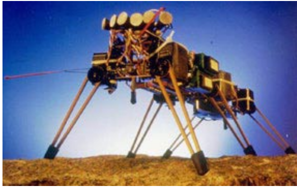
Fig 2.18 Genghis, one of the most famous walking robots from MIT uses hobby servomotors as its actuators ( http://www.ai.mit.edu/projects/genghis )
