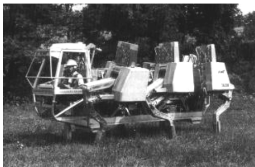
Fig 2.16 The human guided hexapod of Ohio State University
