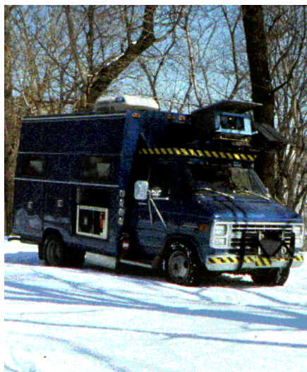
Fig 2.20 Navlab I, the first autonomous highway vehicle that steers and controls the throttle using vision and radar sensors (ROLAND-ref in notes).
