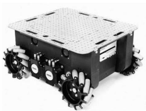
Fig 2.24 The Carnegie Mellon Uranus robot, an omnidirectional robot with four powered swedish 45 wheels.
