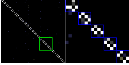
Figure 7: A visualization of the compatibility score matrix obtained for the noise-free case. (left) The entire matrix ( 100 \times 100 ) (right) A zoomed in version of the region marked on the left ( 20 \times 20 ). We observe that a non-zero score is typically assigned only to those pieces that come from the same broken object, even in the presence of several other broken objects.
