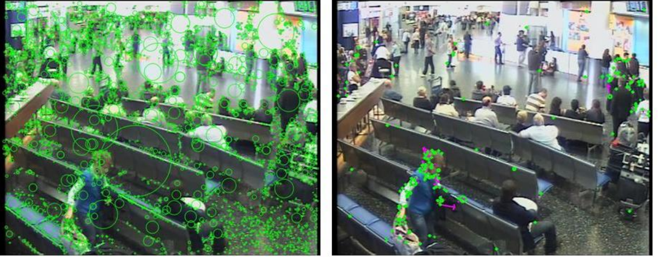
Figure 2: Interest points detected with SIFT (left) and MoSIFT (right). Green circles denote interest points at different scales while magenta arrows illustrate optical flow. Note that MoSIFT identifies distinctive regions that exhibit significant motion, which corresponds well to human activity while SIFT fires strongly on the cluttered background.
