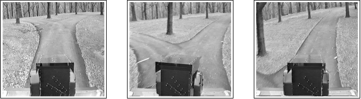
Figure 6: Panacea successfully negotiates a sharp fork in Schenley park. Note the panning of the pan/tilt platform (bottom center) at the intersection to keep the right fork in view.
