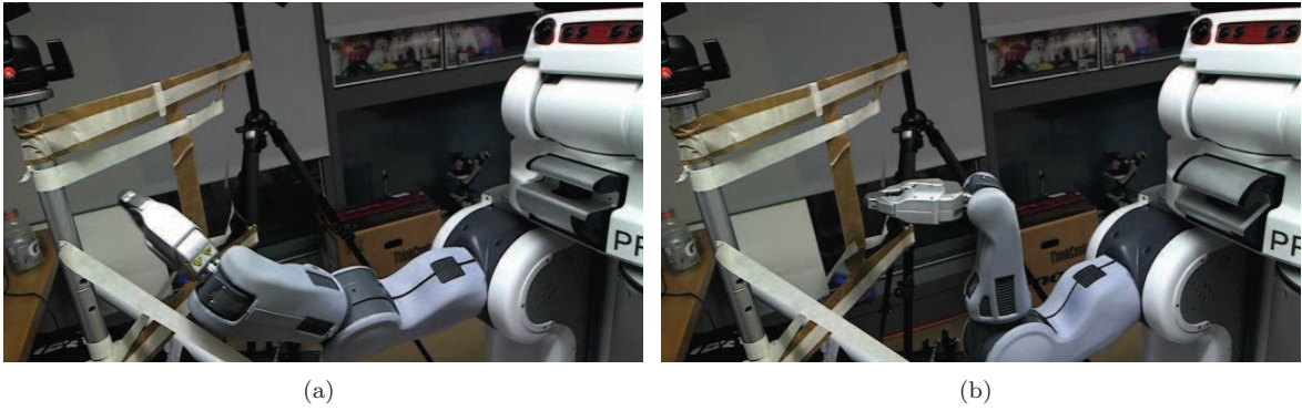
Figure 16: Video stills showing extraneous motions remaining in sampling-based planner's trajectory post-smoothing.
