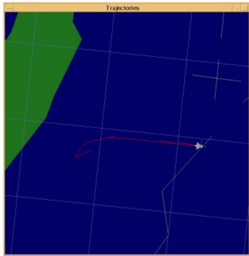
Fig. 5.48: The route taken by the aircraft after the user stepped in and started making high level decisions. Notice the turn to the east near the left of the screen.
