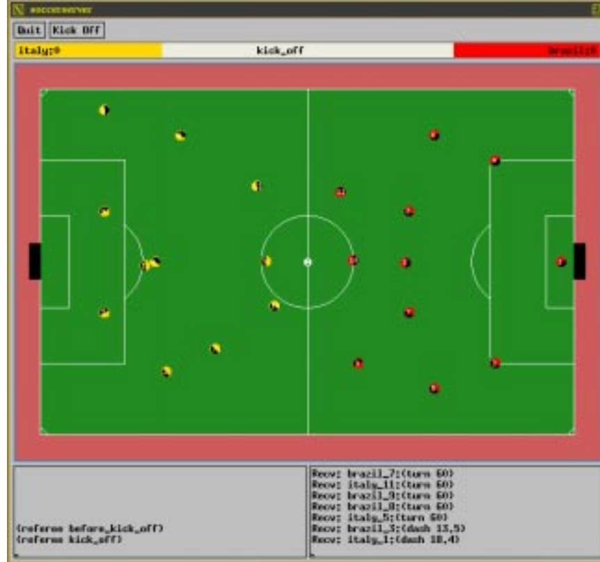
Fig. 5.3: Snapshot of the RoboCup simulation monitor. The larger half light and half dark circles represent the 11 players of each team. The lighter side of the player shows the direction it is facing. In the bottom left hand corner is a record of the commands the automatic referee has sent to the players. In the bottom right hand corner is a record of the commands sent by the players to the server.
