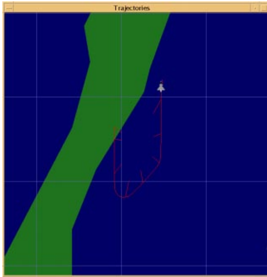
Fig. 5.43: A trace of the path of the aircraft when the location of one of its waypoints is dynamically changed. The “turn” on the right is actually where the waypoint location was changed to be much further north, rather than north-east.
