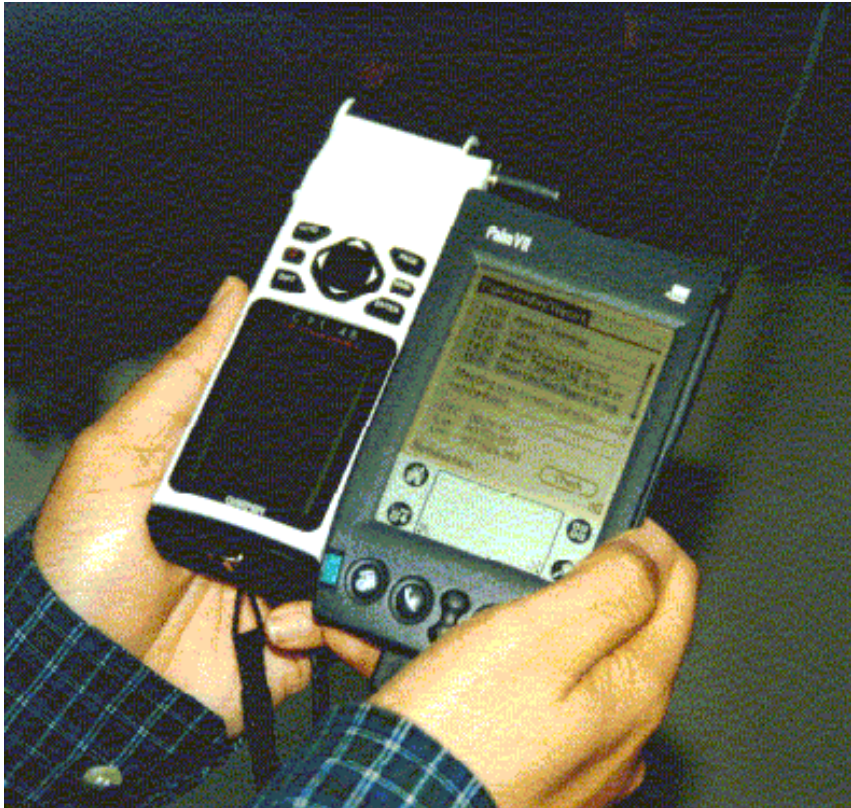
Fig. 6.7: Palm VII connected to GPS device.
