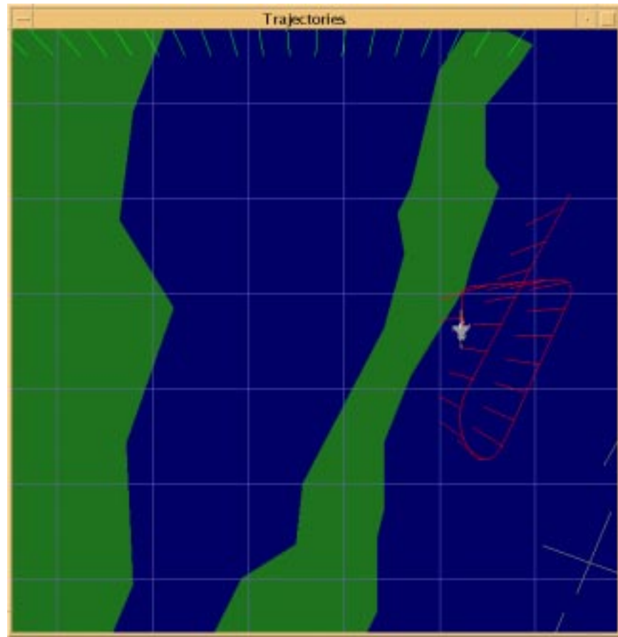
Fig. 5.35: A trace of the aircraft's path during the patrol. The turn at the bottom (one long turn) was made while the Smooth Manager was active and the tighter turn at the top was made while the Smooth Manager was paused.
